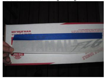
5. Now take your finger or thumb and rub all around with some pressure to make sure every thing is good and stuck. Begin removing the transfer tape starting at a top corner and pulling it "low" meaning keep the tape close to the surface instead of pulling straight out towards you. Don't forget to remove the clear transfer tape that is a layer under the paper tape that I have to use to be able to see through when I am layering the colors.
