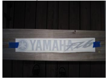
2. Next run a piece of masking tape along the top edge as I show from one end to the other and securely lock the top of the decal to the swingarm. This is called the hinge meathod and it works great.
